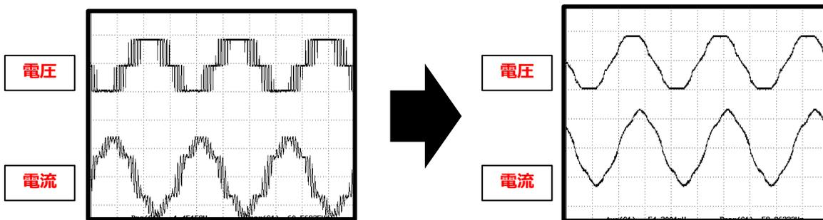
$F_c = 5\text{kHz}$ , output = 50Hz, 80% load
